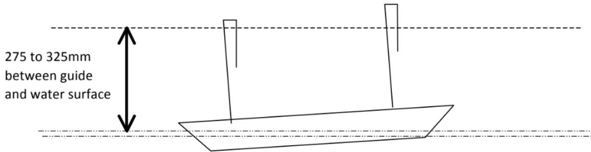
Figure 2 – Guide line height and suggested guide rod position
