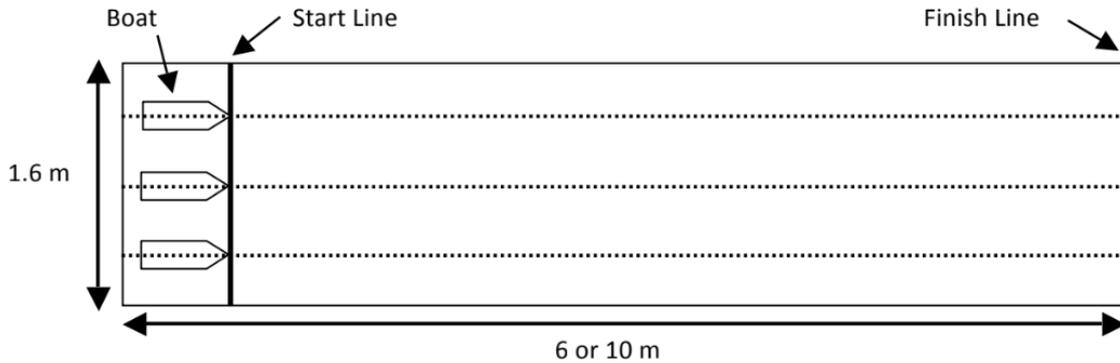
Figure 1 – Layout of a pool configured for three (3) lanes with boats at the starting line
